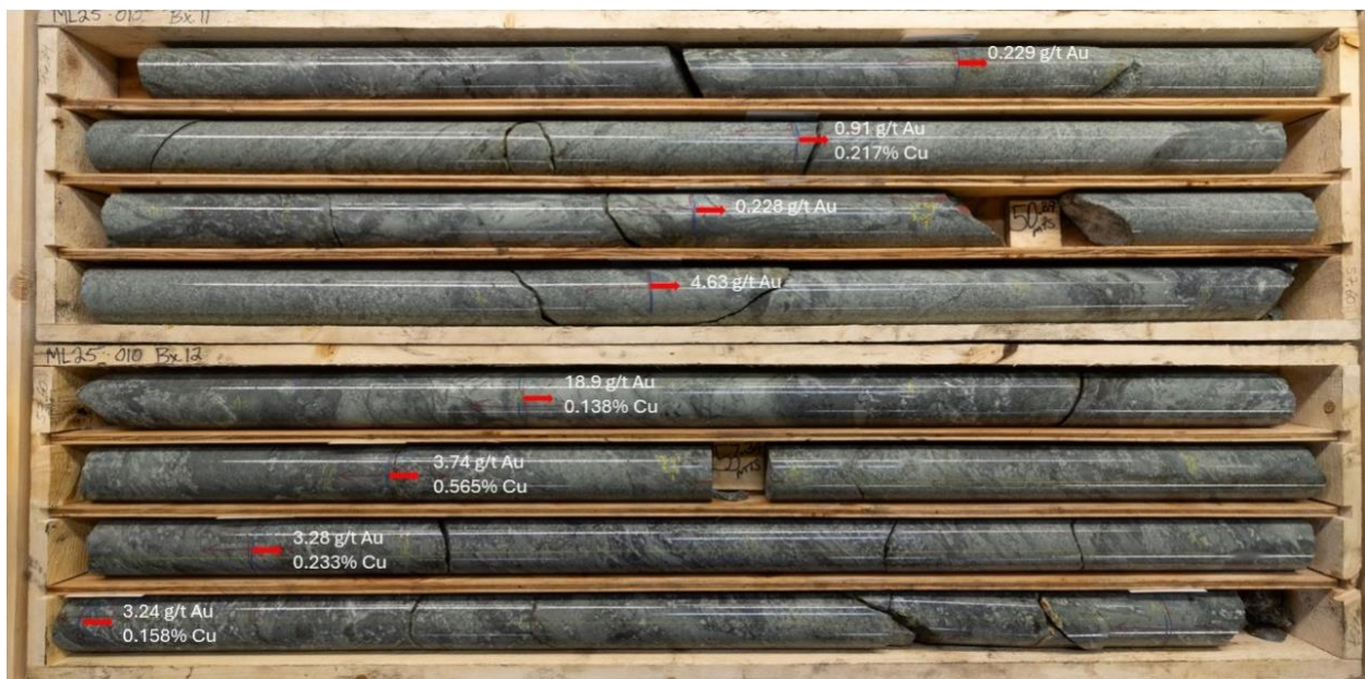
Figure 3: ML25-010 from 42.24 – 56.07m with gold and copper assays. Red arrows mark the beginning of the sampled interval.
